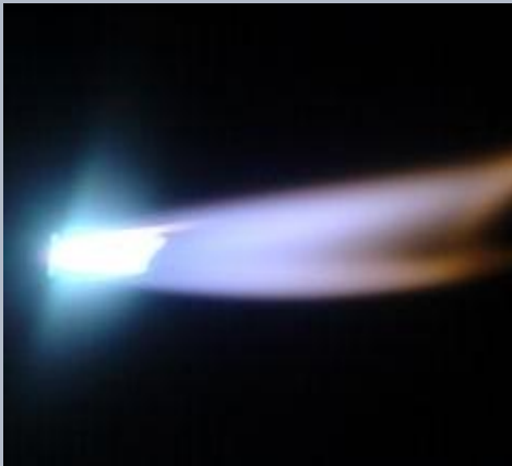
The acetylene-oxygen flame (a temperature of about 2621 °C in 2-3 mm from the core)
