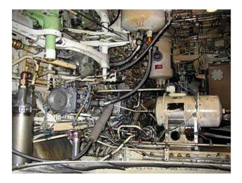
THE BOEING 737 HAS THREE HYDRAULIC SYSTEMS: A, B (MAIN) AND STANDBY (STANDBY). AT 737-100 AND -200, SYSTEM A **OPERATES ON TWO MOTOR** PUMPS, AND SYSTEM B OPERATES ON TWO ELECTRIC PUMPS. THE **BACKUP SYSTEM IS POWERED BY** A RECHARGEABLE BATTERY AND ONLY SUPPLIES THE SLATS, **RUDDER AND REVERSE. MOST** HYDRAULIC COMPONENTS ARE LOCATED IN THE CHASSIS NICHE.
