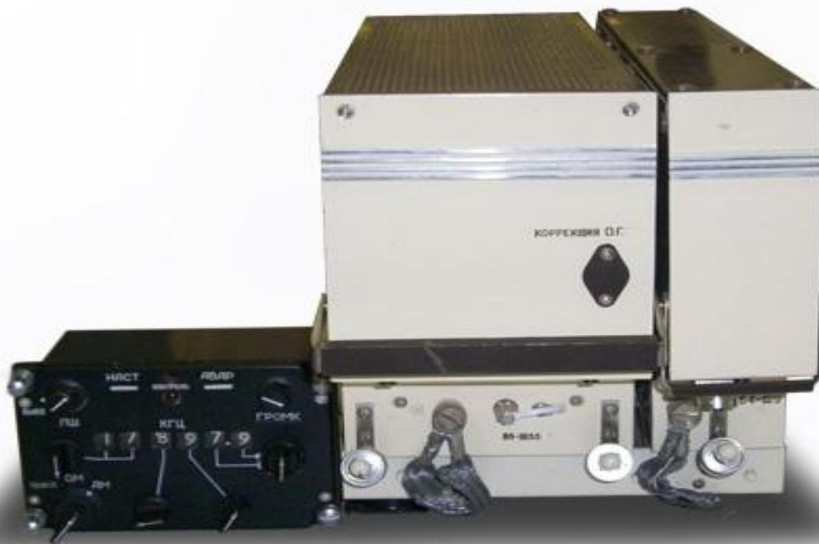
Radio control is carried out from the remote control. The radio is powered by a direct current from the battery bus through the automatic circuit breaker of the AZSGK-25-2s “SVYAZN RS” network, located on the left panel of the electric panel gas station.
