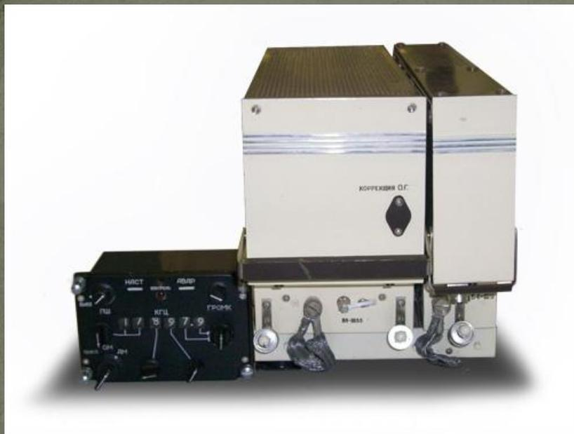
The radio station is structurally made on the block principle. All units of the radio station, except for the remote control (RC), are located in the radio compartment between frames No. 13 and 16.
