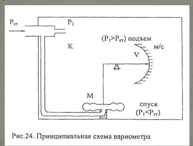
This division of the body of the device into two sections is made in order that the heat released during the operation of the gyromotor does not affect the operation of the variometer due to changes in the pressure of the PCT in the body of the device.
