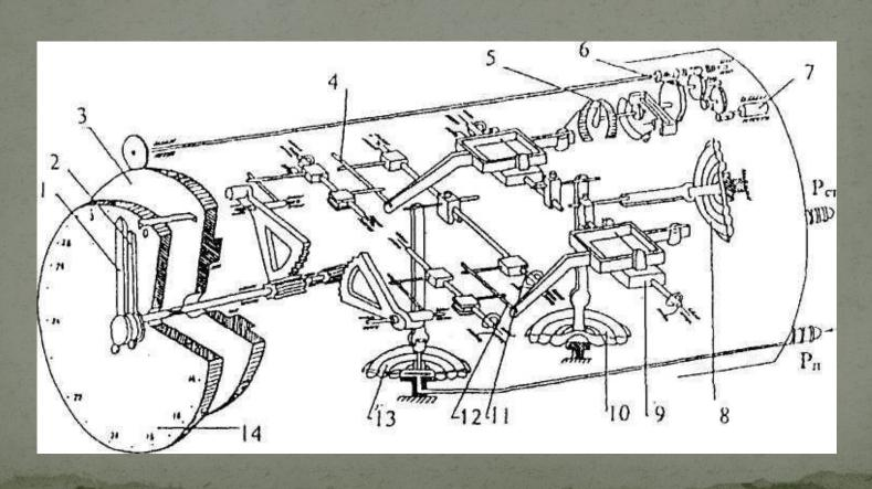
manometric box 10, the inner cavity of which is connected to the atmosphere through the pipeline 9 and the nozzle 8 through the static wiring of the helicopter (PVD-6).
