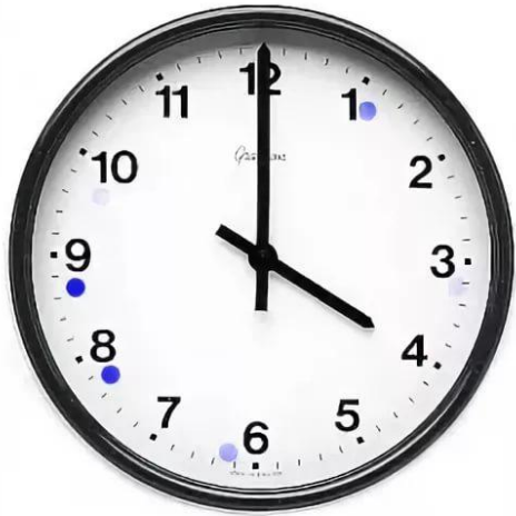
Each LED (blue dot) represents a level of color intensity, this being the LED's level of brightness and amount of presence detected per hour. As you can see, hours 1, 8 and 9 have a heavy presence detected, whereas 3, 6 and 10 had minima contact.
