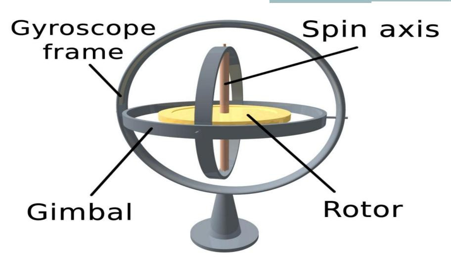
Gyroscope- is a device used for measuring or maintaining orientation and angular velocity.
