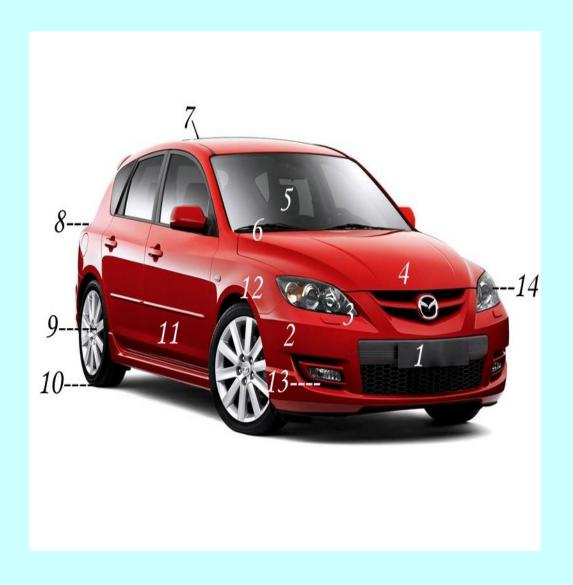
fog light, brake light, rear light, hood, headlight, hubcap, tire, bumper, windscreen, windscreen wiper, door, number plate, wing, antenna,
