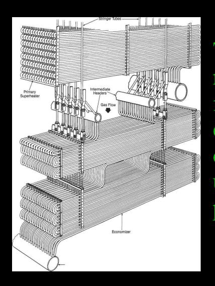
The economizer is a mechanical device intended to reduce energy consumption, or to perform another useful function like preheating fluid.
