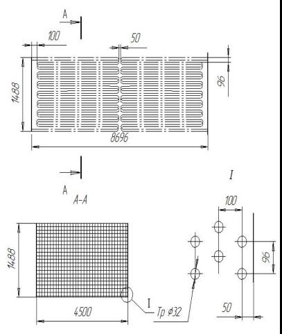
Boiler economizers are series of horizontal tubular elements generally made from low-carbon steel.
