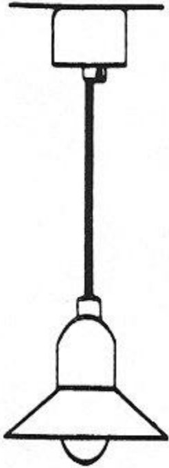
Pendant, or Fixture Wiring
