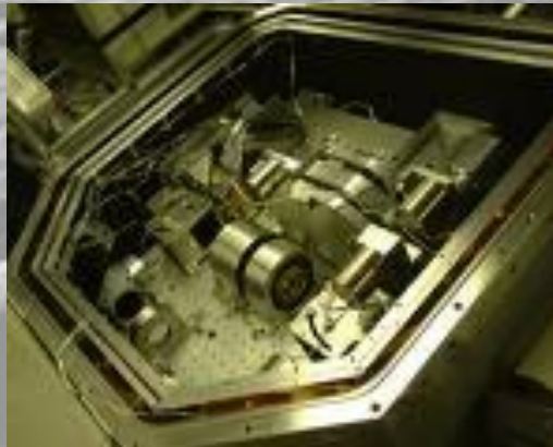
Subaru's primary near-IR camera & Spectrograph
