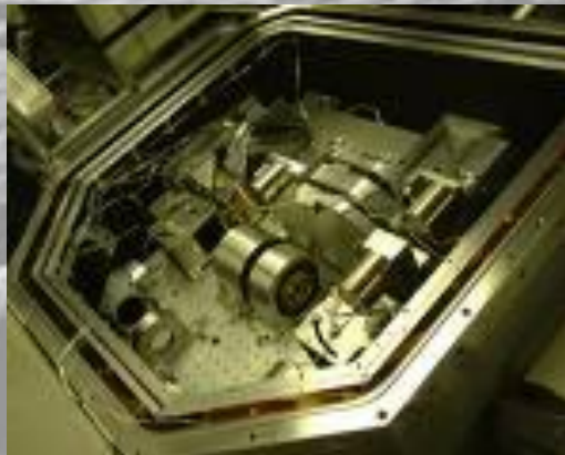
Subaru's primary near-IR camera & Spectrograph
