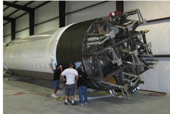
First stage mated with thrust frame
