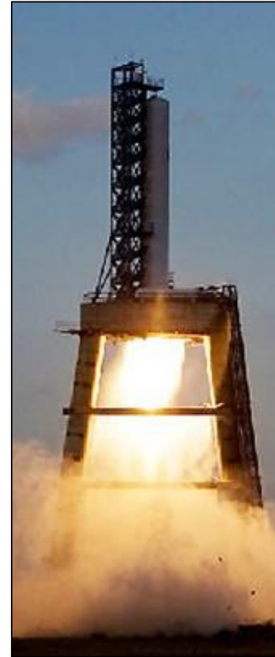
1 st stage test firing with multiple engines
