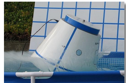
1:3 scale Model Splash Test
