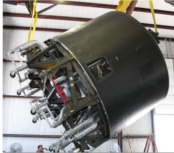
Thrust frame & plumbing for nine engines
