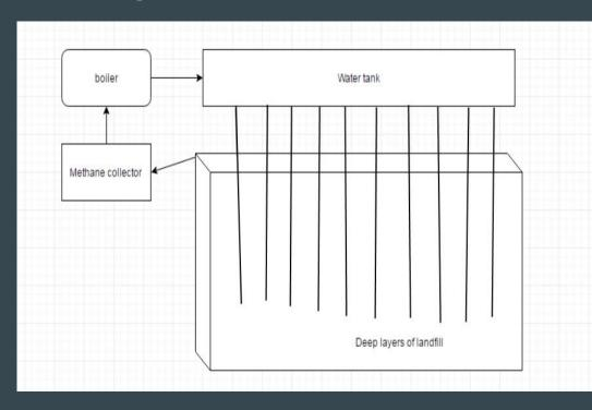
Using the methane created by waste we can increase the temperature of deep layers.
