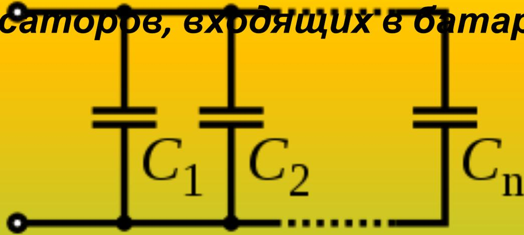
$$C = C_1 + C_2 + \dots + C_n$$
