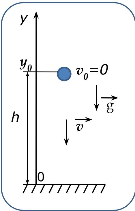
$$s_y = v_{0y} t + g_y t^2 / 2 \quad -h = -g_y t^2 / 2$$
