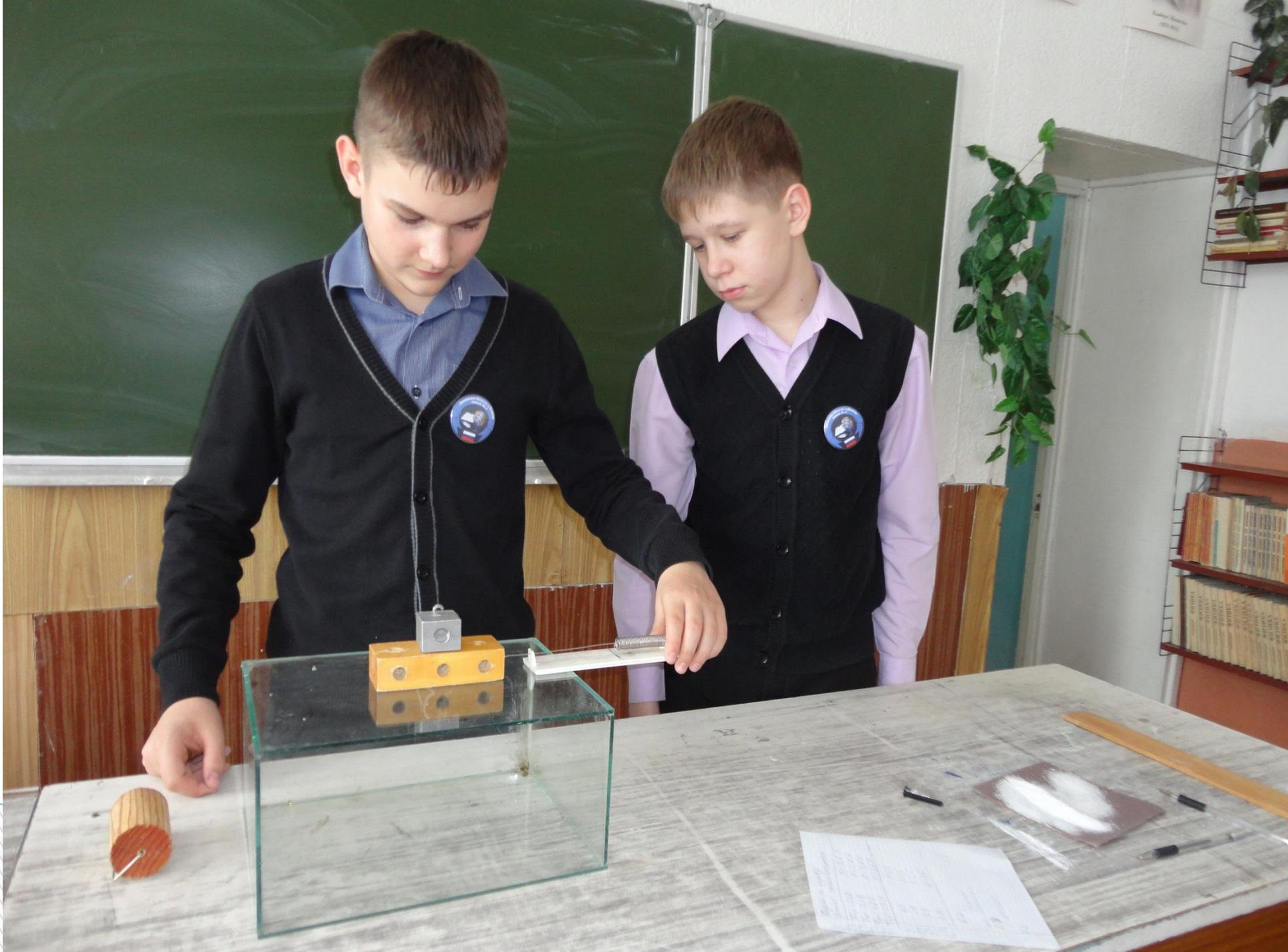
The boy on the left is wearing a black cardigan over a blue shirt. The boy on the right is wearing a black vest over a light purple shirt. Both are wearing blue circular badges. They are using a glass tank, a yellow wooden block, a metal weight, and a spring scale to measure buoyant force.
