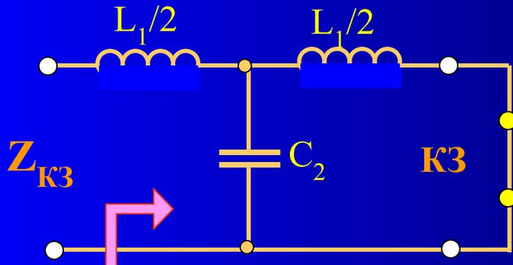
$$Z_{K3}(p) = \frac{pL_1}{2} + \left(pC_2 + \frac{2}{pL_1}\right)^{-1} = \frac{pL_1(p^2 L_1 C_2 + 4)}{2(p^2 L_1 C_2 + 2)}$$
