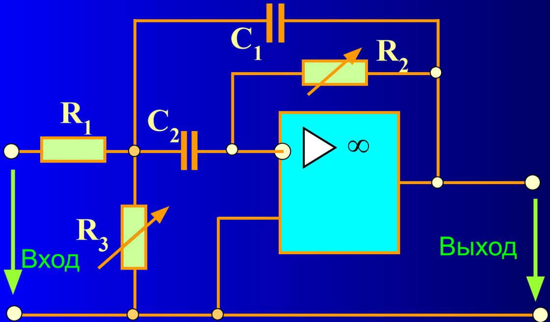
$$f_0 = \frac{1}{2\pi} \sqrt{\frac{1 + \frac{R_1}{R_3}}{1 + \frac{C_2}{C_1}}}$$
