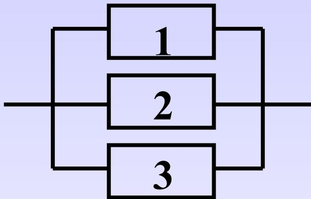
$$I_{\text{общ}} = I_1 + I_2 + I_3 + \dots \quad \left( I = \frac{q_0 N}{\Delta t} \right)$$
