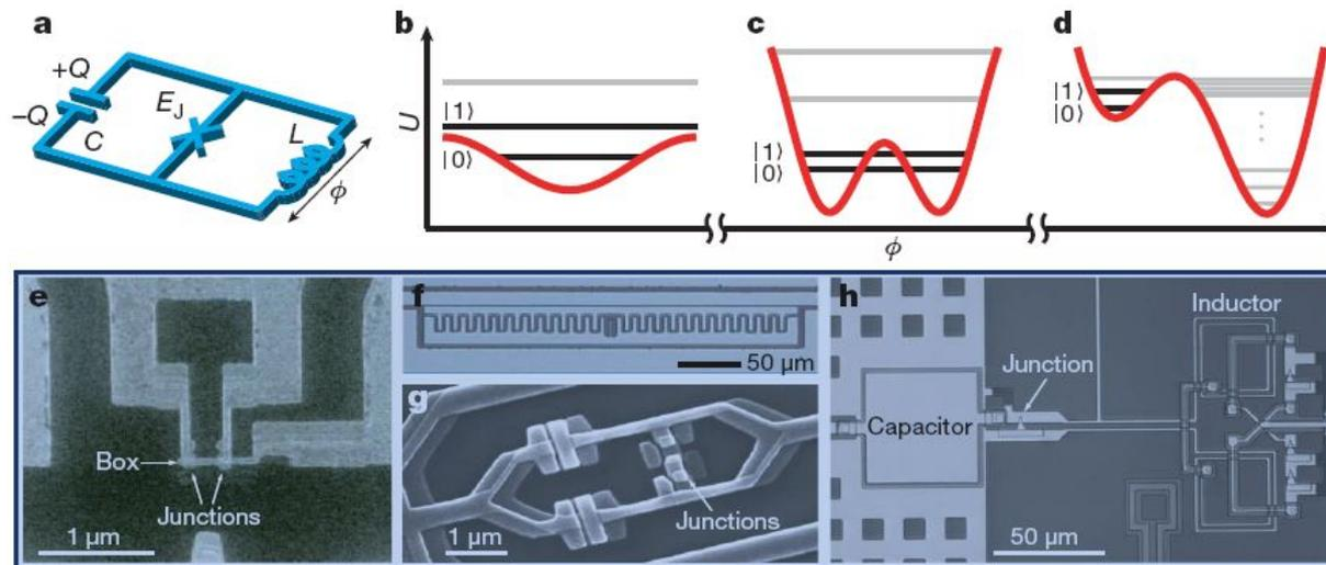
**Figure 5 | Superconducting qubits.** **a**, Minimal circuit model of superconducting qubits. The Josephson junction is denoted by the blue 'X'. **b–d**, Potential energy  $U(\Phi)$  (red) and qubit energy levels (black) for charge (**b**), flux (**c**), and phase qubits (**d**), respectively. **e–h**, Micrographs of superconducting qubits. The circuits are made of Al films. The Josephson
