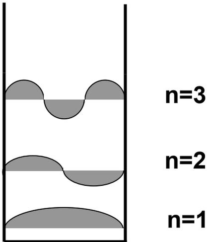
$$\psi_{n(c,v)} \equiv \begin{cases} \sqrt{\frac{\Omega}{V}} \sin\left(\frac{n\pi}{L_z} z\right) \exp\left(ik_{\parallel} r_{\parallel}\right) u_{c,v}(r) & - \text{ В яме} \\ 0 & - \text{ вне ямы} \end{cases}$$
