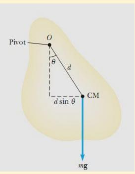
If a hanging object oscillates about a fixed axis that does not pass through its center of mass and the object cannot be approximated as a point mass, we cannot treat the system as a simple pendulum. In this case the system is called a physical pendulum.
