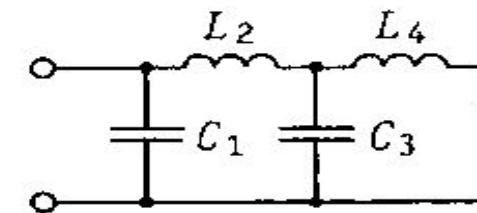
$C_1 = 1,0 \text{ мкФ}; L_2 = 20 \text{ мГн}; C_3 = 1,04 \text{ мкФ}; L_4 = 9,4 \text{ мГн}.$
