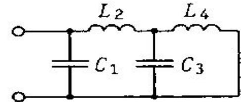
$$C1 = 1,0 \text{ мкФ}; L2 = 20 \text{ мГн}; C3 = 1,04 \text{ мкФ}; L4 = 9,4 \text{ мГн}.$$
