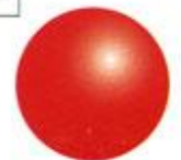
Diameter 0.5 mm Uranium dioxide Fuel
