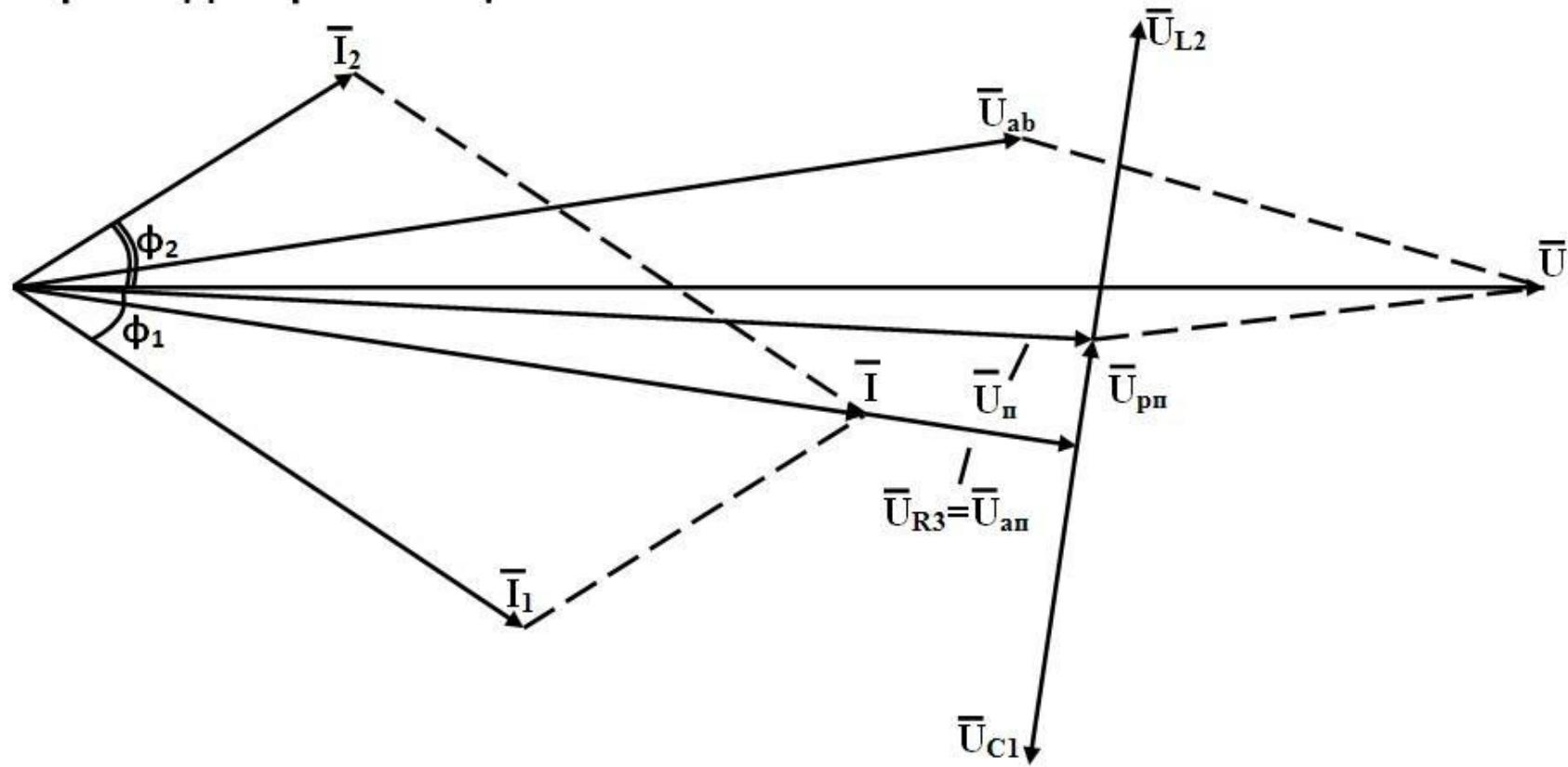
**Где**  $\varphi_1 = \arctg \frac{X_{L1}}{R_1}$ ,  $\varphi_2 = \arctg \frac{X_{C2}}{R_2}$ ,  $U_{R3} = IR_3$ ,  $U_{L2} = IX_{L2}$ ,
