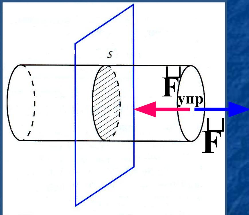
$$\sigma = \frac{F_{\text{упр}}}{S} \quad [\sigma] = \frac{\text{Н}}{\text{м}^2} = \text{Па}$$
