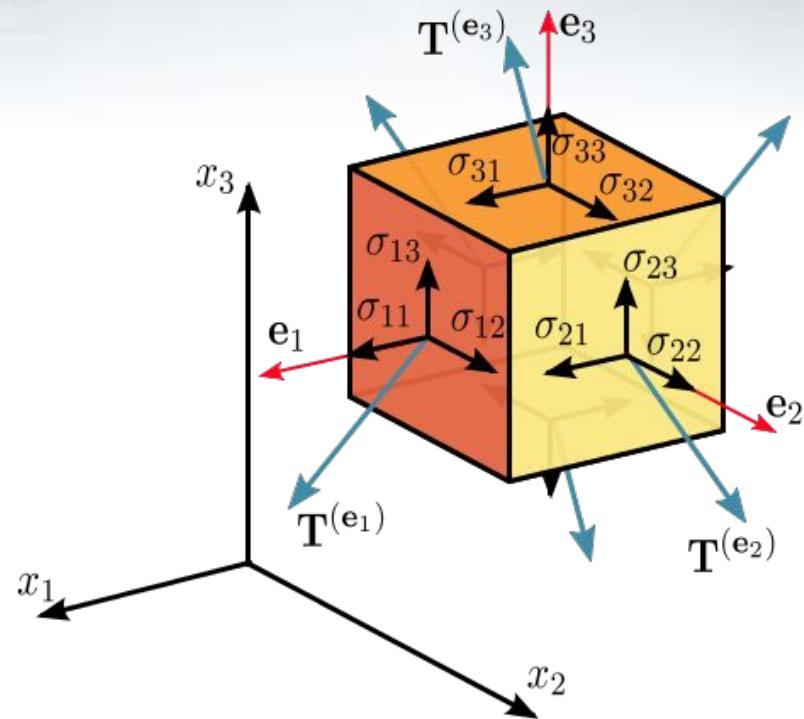
$$\boldsymbol{\sigma} = \begin{bmatrix} \sigma_{11} & \sigma_{12} & \sigma_{13} \\ \sigma_{21} & \sigma_{22} & \sigma_{23} \\ \sigma_{31} & \sigma_{32} & \sigma_{33} \end{bmatrix} \equiv \begin{bmatrix} \sigma_{xx} & \sigma_{xy} & \sigma_{xz} \\ \sigma_{yx} & \sigma_{yy} & \sigma_{yz} \\ \sigma_{zx} & \sigma_{zy} & \sigma_{zz} \end{bmatrix} \equiv \begin{bmatrix} \sigma_x & \tau_{xy} & \tau_{xz} \\ \tau_{yx} & \sigma_y & \tau_{yz} \\ \tau_{zx} & \tau_{zy} & \sigma_z \end{bmatrix}$$
