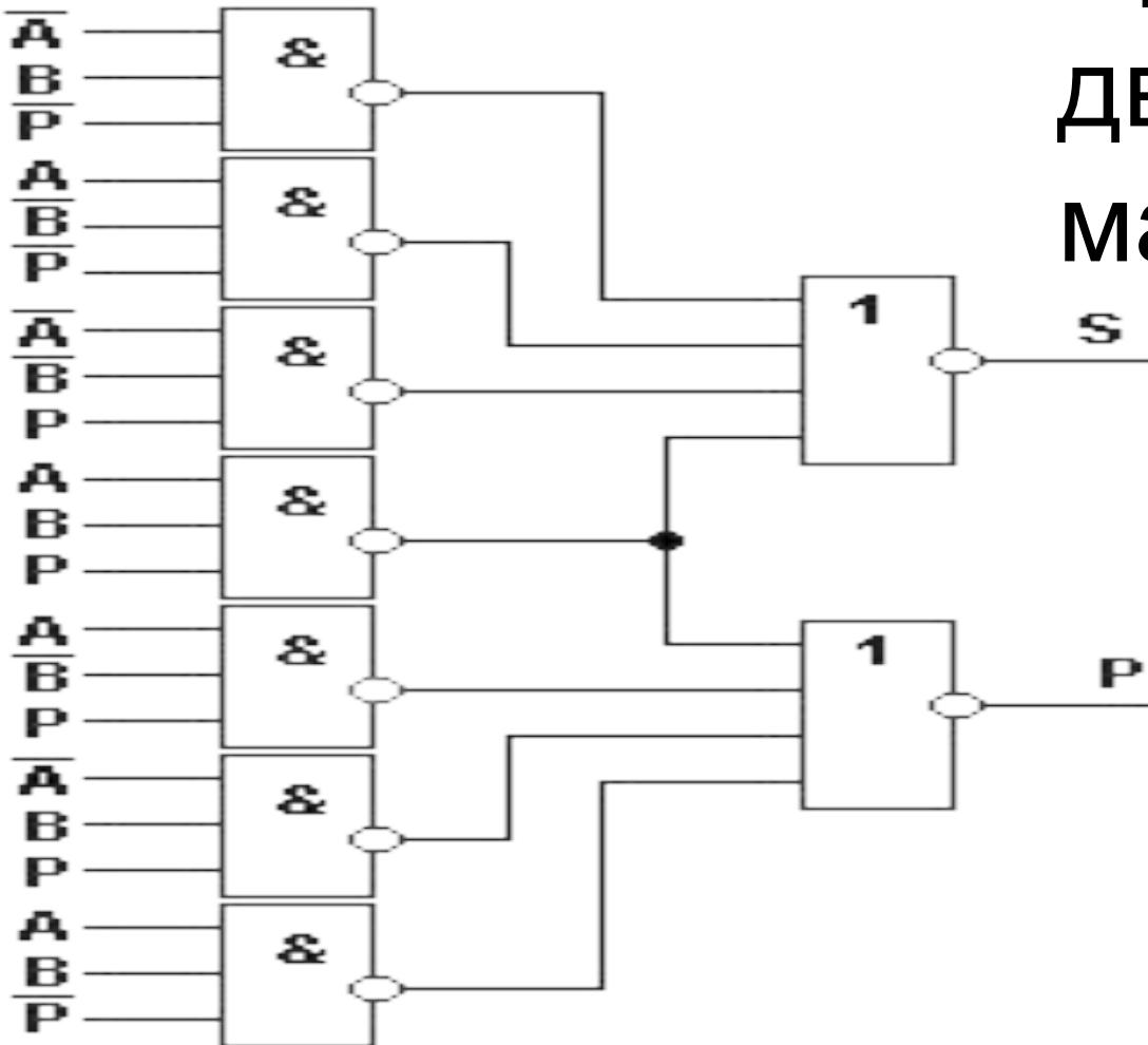
$\blacksquare \quad S = A\overline{BP} \vee \overline{AB}\overline{P} \vee \overline{AB}P \vee ABP$
