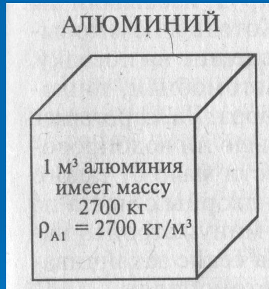
$$\rho_{ал} = 2700 \frac{\text{кг}}{\text{м}^3} = 2700 \times \frac{1000\text{г}}{1000000\text{см}^3} = 2,7 \frac{\text{г}}{\text{см}^3}$$
