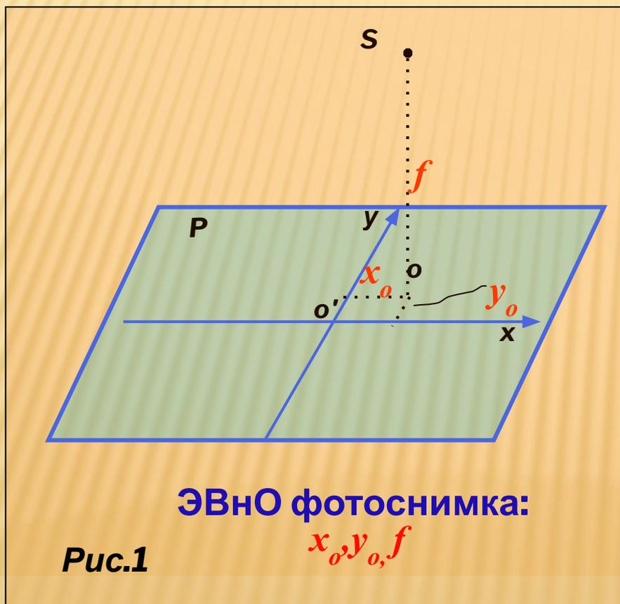
$$\left. \begin{aligned} x &= x' - x_0 \\ y &= y' - y_0 \end{aligned} \right\} (1.6)$$
