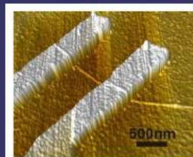
SWNT Diameter: 1.7 and 2.2nm Device length: 600nm
