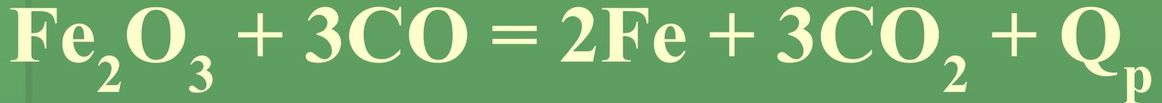
$$Q_p = 3Q_{\text{обр}}(\text{CO}_2) - [3Q_{\text{обр}}(\text{CO}) + Q_{\text{обр}}(\text{Fe}_2\text{O}_3)] = 3 \cdot 394 - [3 \cdot 110 + 820] = 32 \text{ кДж}$$
