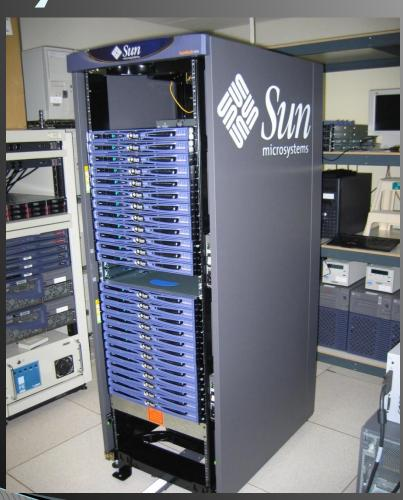
A computer cluster consists of a set of loosely or tightly connected computers
