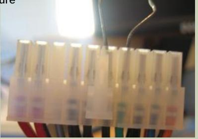
Next, put your paperclip into the pin with the green wire and the other end into one of the two black ground wires beside the green wire. With your teachers permission power on the
