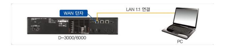
When you use one D-3000 device, it is recommended to connect the device with PC/laptop and use extra network router.
