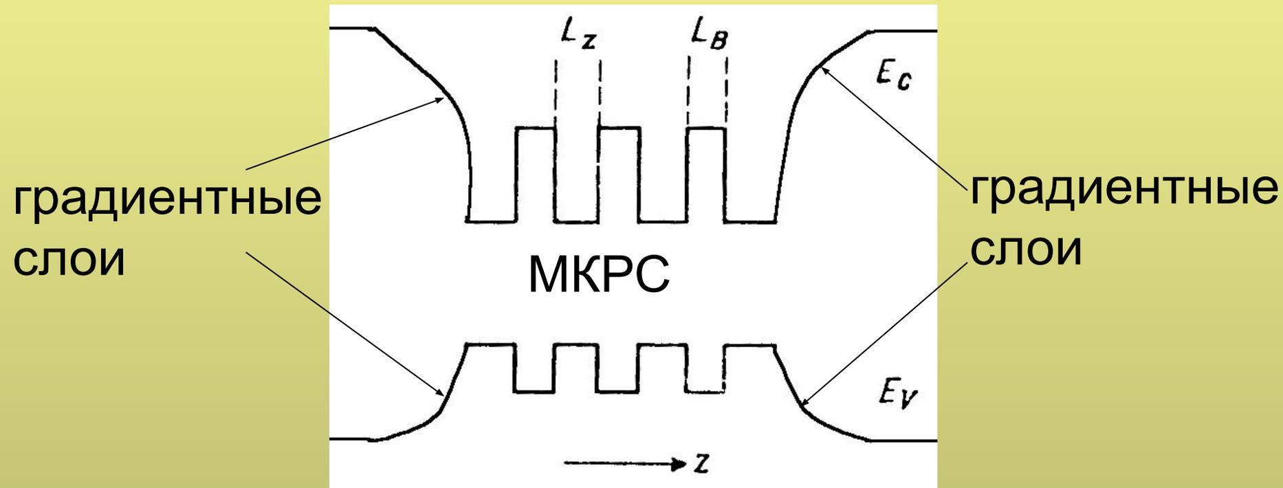
graded-index separated confinement heterostructure
