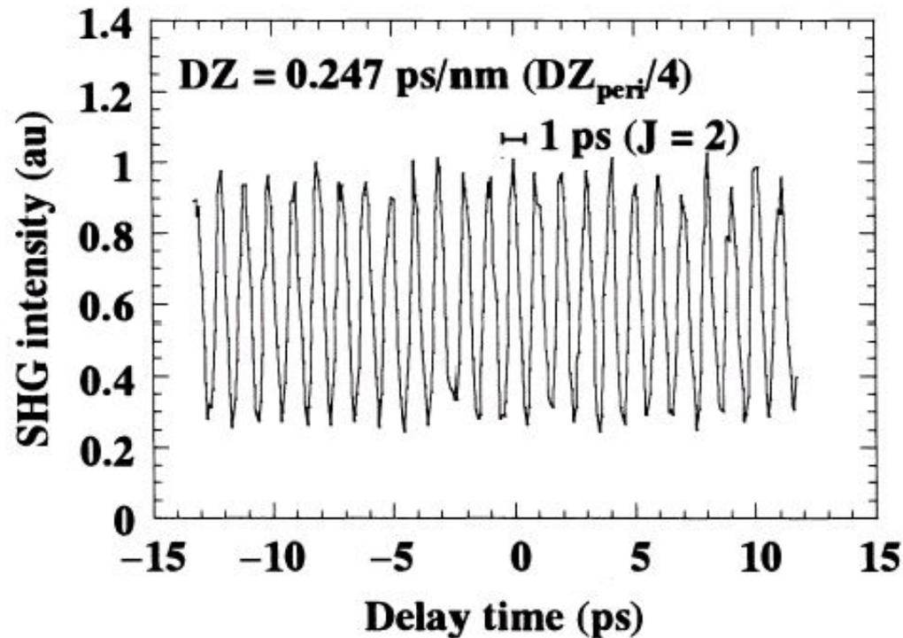
SHG correlation trace of 1 THz optical pulse train obtained by two-times multiplication of a 500-GHz CPM-LD.
