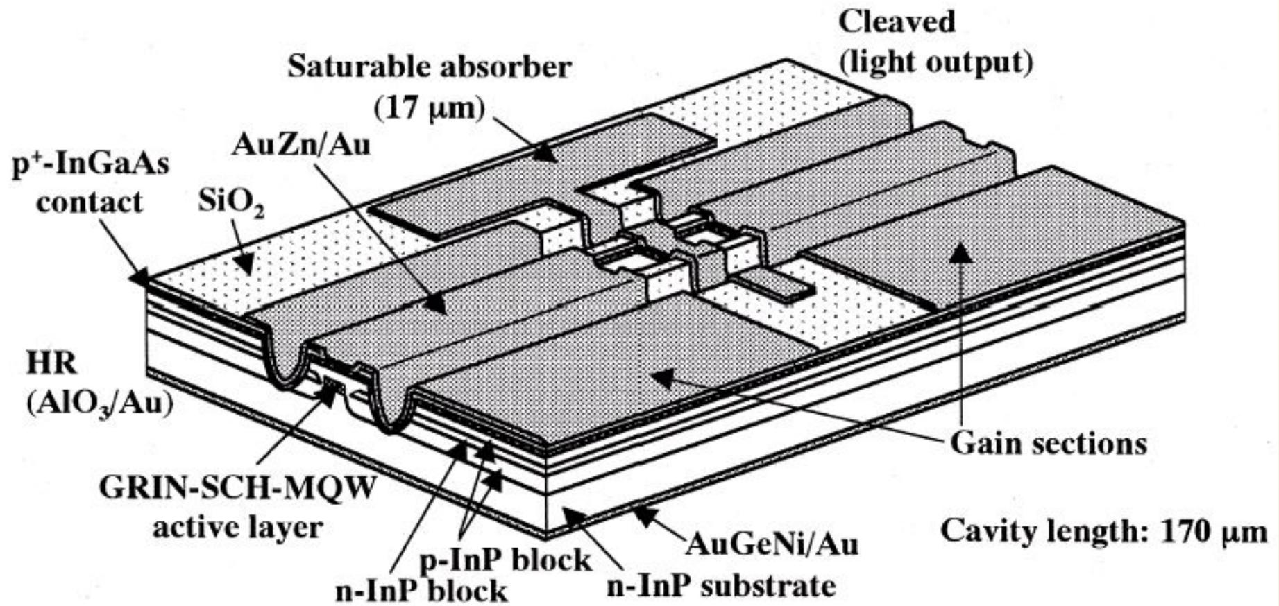
Device structure of a short-cavity GRIN-SCH-MQW CPM-LD.
