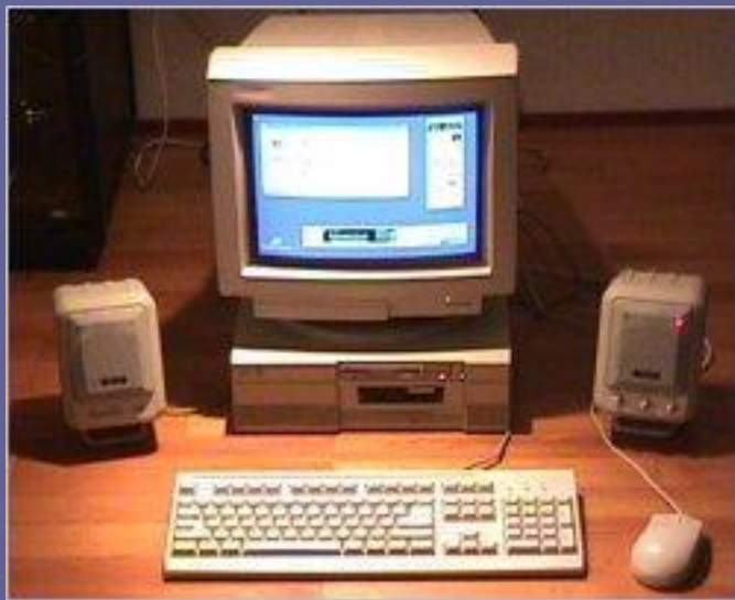
Intel 80386SX + 80387SX, 20 MHz 4 MByte Expandable up to 16 MByte 102 MB Hard disk
