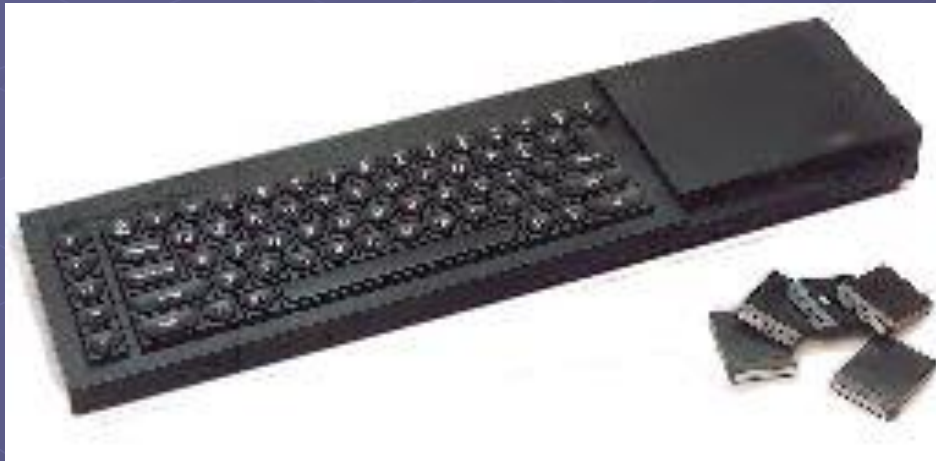
Sinclair QL Printer, TV as monitor Motorola 68008 at 7.5MHz, 128k RAM (Max 640k) 32k ROM
