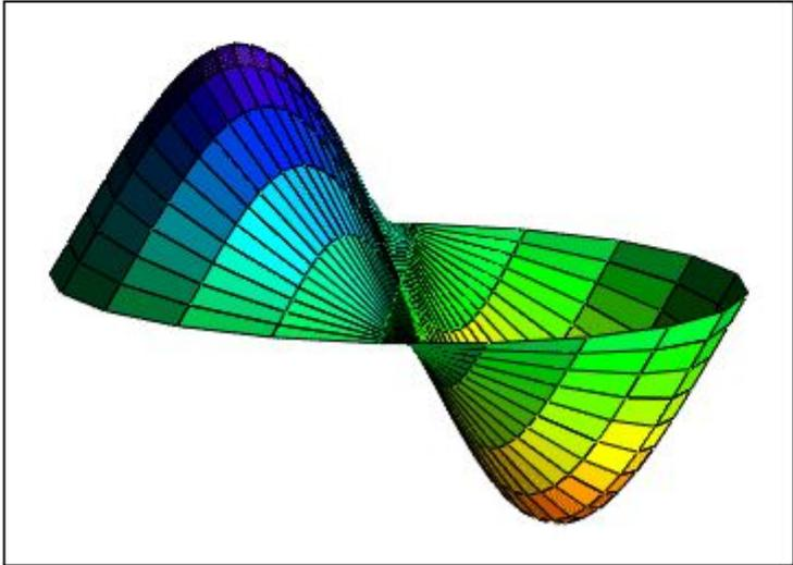
A 3D surface plot showing the deformation of a drum's surface over time. The surface is colored with a gradient from purple (high) to green (low), and is shown in a perspective view. The plot illustrates a complex, multi-lobed shape, characteristic of a higher-order mode of vibration.
