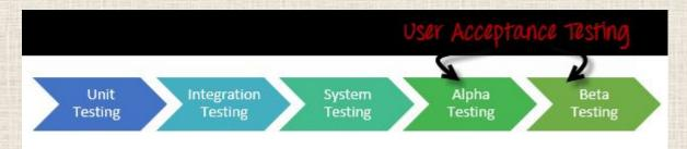
**<u>Beta testing</u>** also known as user testing takes place at the end users site by the end users to validate the usability, functionality, compatibility, and reliability testing.
