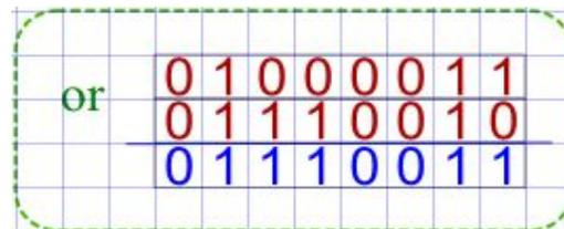
Diagram illustrating the bitwise OR operation. The first number (67) is 01000011 and the second number (114) is 01110010. The result is 01110011. The operation is labeled 'or'.
