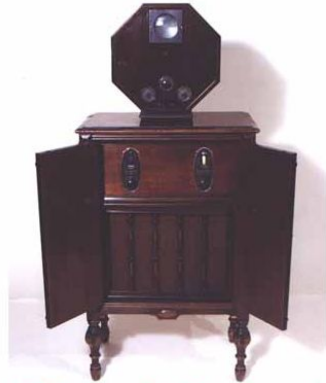
1928 G.E. Scanning Disk Television Set (closed-open)
