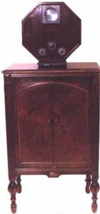
1928 G.E. Scanning Disk Television Set (closed-open)
