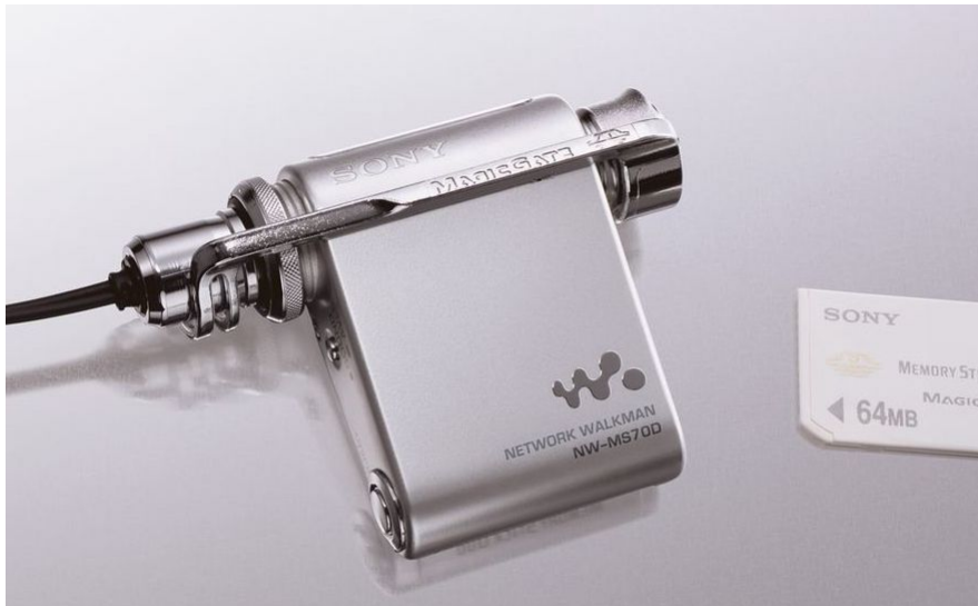
began using flash memory in the early 2000s. This 2003 Walkman features both 256 MB of built-in flash memory and
