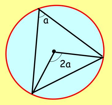
The angles made at the centre of the circle is double the angle made at the edge of the circle from the same two points (two ends of the chord)
