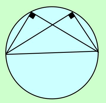
A triangle drawn from <u>the two ends of a</u> <u>diameter</u> will <u>ALWAYS</u> make an angle 90° where it hits the edge of the circle.
