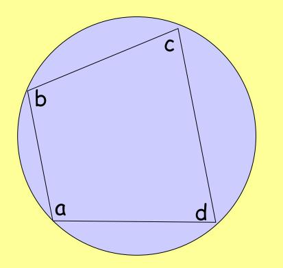
A cylclic quadrilateral is a 4-sided shape with every corner touching the circle. Both pairs of opposite pairs of angles add up to 180°
