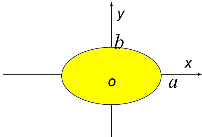
$$\begin{aligned} S &= 4 \int_0^{\pi/2} b \sin t (-a \sin t) dt = \\ &= 4ab \int_0^{\pi/2} \sin^2 t dt = 4ab \int_0^{\pi/2} \frac{1 - \cos 2t}{2} dt = \\ &= \frac{1}{2} 4ab \left( t - \frac{1}{2} \sin 2t \right) \Big|_0^{\pi/2} = 2ab \frac{\pi}{2} = \pi ab. \end{aligned}$$
