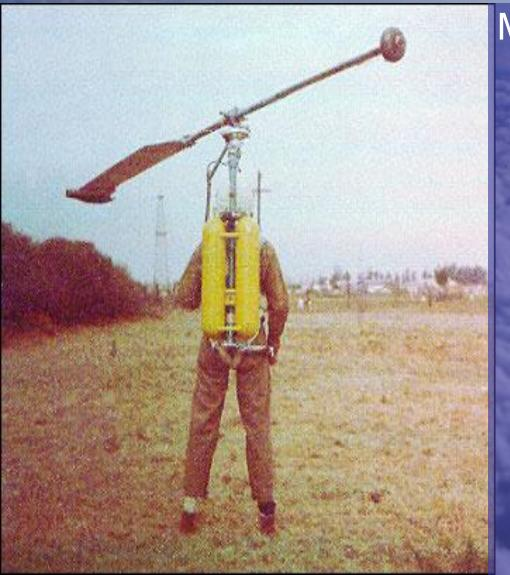
MEG-1X was created by American engineer Eugene Gluhareff in 1955. The creator of MEG-1X, following the ancient wisdom "the less, the better", has coherently thrown out all the excessive details, he did not spare even the blades: only one of them stayed with a jet engine, attached to its end.
