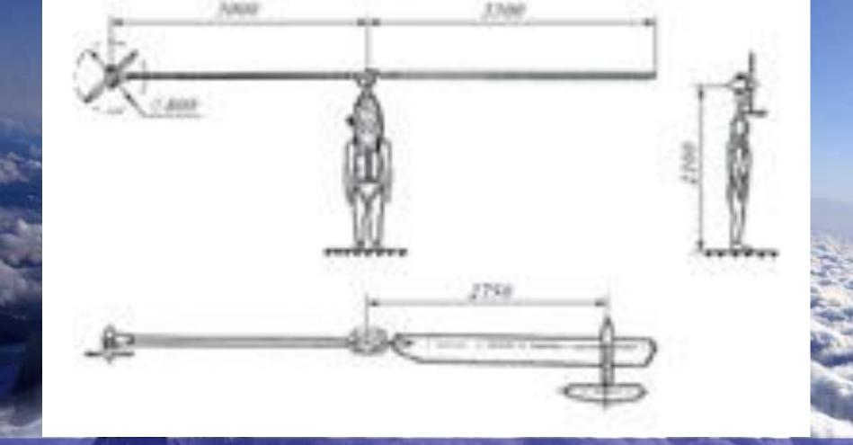
In USSR the pioneer in creation of single bladed helicopter was the student of Kharkov Aviation Institute, Yuri Marinchenko. The original version of helicopter was planned as a backpack weighting 30 kg. He developed this idea during a year and, in 1971 the model was established.
