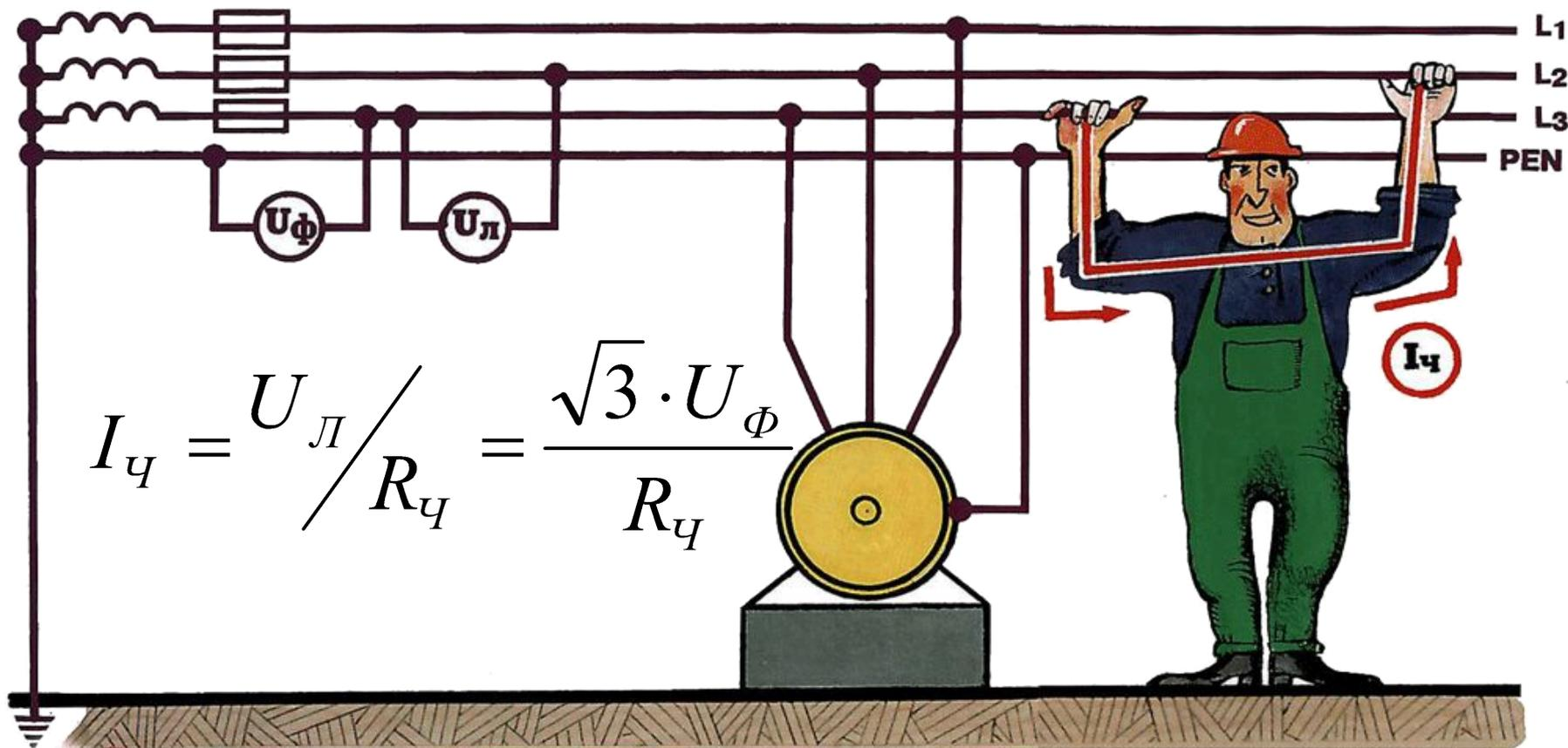
$$I_{\text{ч}} = \frac{U_{\text{л}}}{R_{\text{ч}}} = \frac{\sqrt{3} \cdot U_{\text{ф}}}{R_{\text{ч}}}$$
