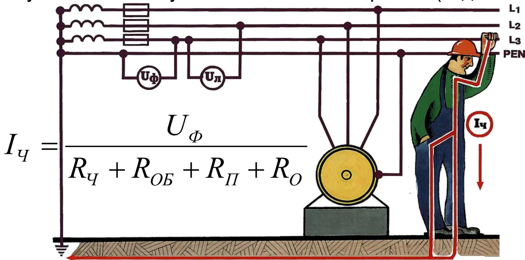
$$I_\lambda = \frac{U_\phi}{R_\lambda + R_{OB} + R_\Pi + R_O}$$
