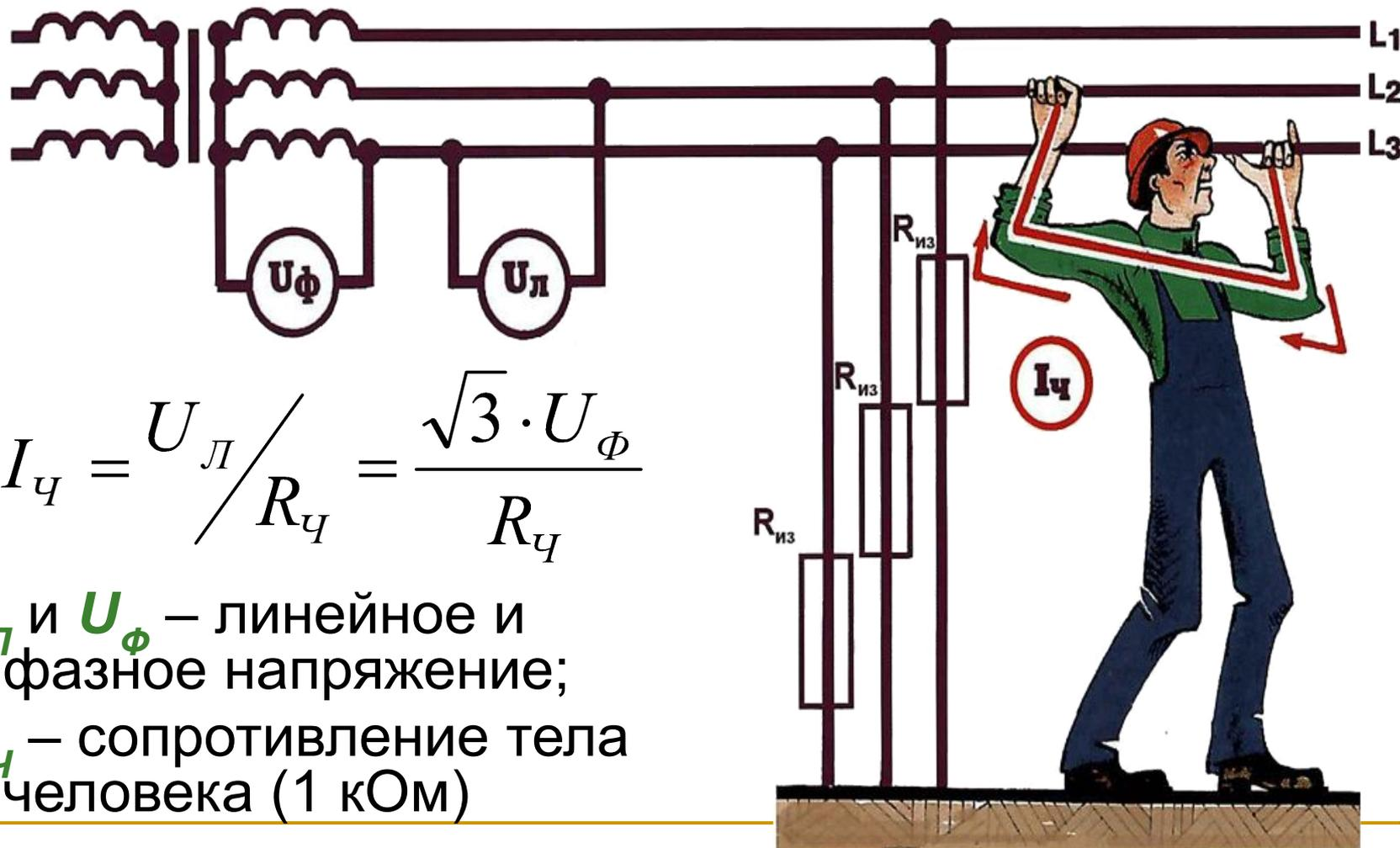
$$I_{\text{ч}} = \frac{U_{\text{л}}}{R_{\text{ч}}} = \frac{\sqrt{3} \cdot U_{\text{ф}}}{R_{\text{ч}}}$$
