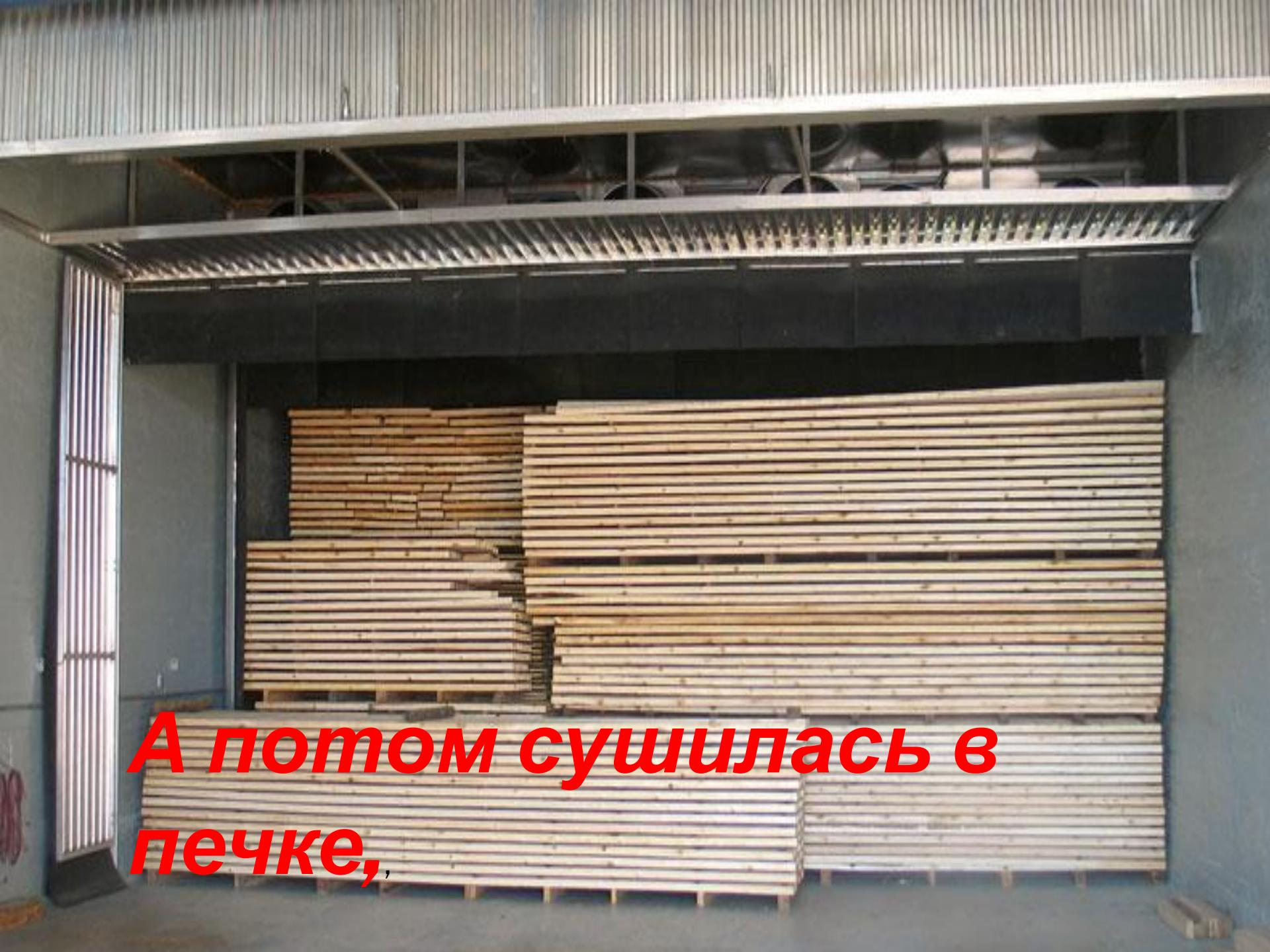
A photograph of a large industrial kiln or oven. The interior is filled with numerous wooden logs stacked in several rows. The kiln has a dark, metallic exterior with a large door on the left side. Above the kiln, there is a complex system of metal pipes and ducts, likely for ventilation and heating. The lighting is somewhat dim, coming from within the kiln and some overhead lights.
