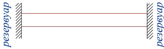
$$J_i = ev_i \delta n_i = e \frac{1}{\hbar} \frac{\partial \epsilon}{\partial k} eV \frac{\partial n}{\partial \epsilon} = \frac{e^2}{\hbar} \frac{\partial \epsilon}{\partial k} \frac{\partial n}{\partial \epsilon} \frac{\partial k}{\partial \epsilon} V$$
