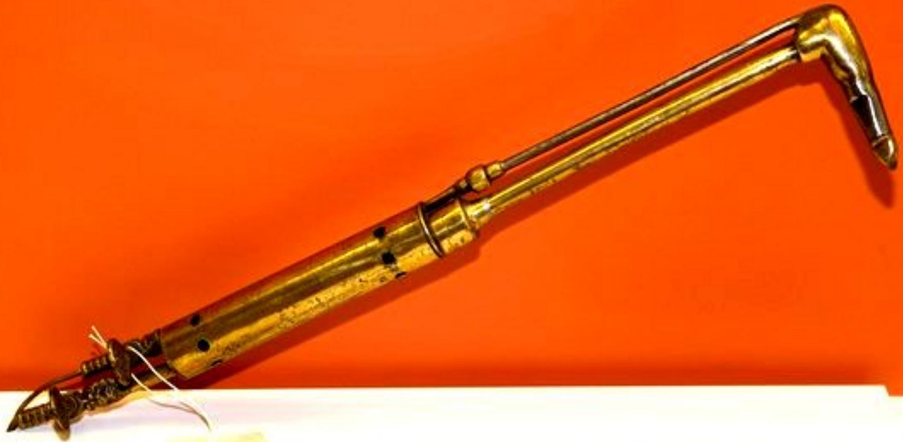
Torch for oxy-acetylene welding
