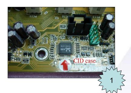
Visual Inspection to check Audio connector, Audio chip & nearby related components are not damaged.
