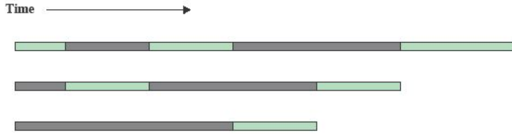
(a) Interleaving (multiprogramming, one processor)
