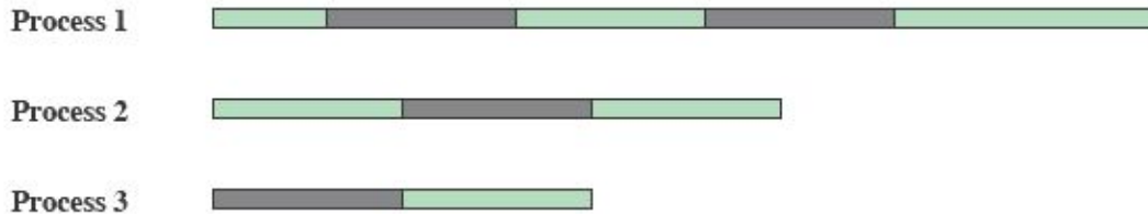
(b) Interleaving and overlapping (multiprocessing; two processors)
